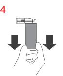
Examine the new reload for the presence of a staple retaining cap. Remove the staple retaining cap by sliding it off the reload. If the retaining cap is not in place, discard the reload.
