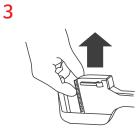
Remove the used reload from the instrument. Grasp the top of the reload and lift upward, unsnapping the reload from the jaws. Properly discard the used reload.
